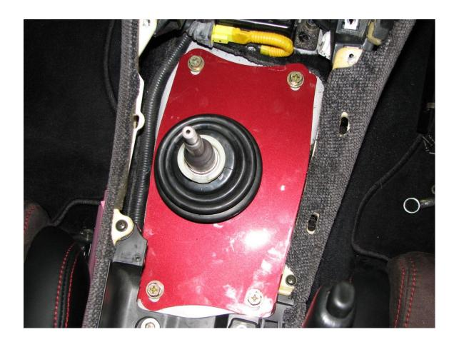
If you purchased the *Zspeed* upgraded tunnel boot plate with your new solid shift mount simply slide over shifter and carefully roll the top of the boot over the shift knob stop plate being careful not to rip boot. A little lube helps getting it over the shift knob stop plate.
