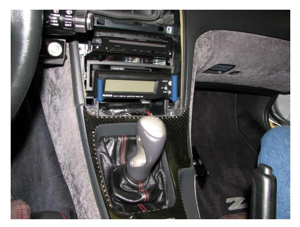
Radio trim removed, Remove 3 screws from shifter trim. The other screw is under the ash tray. Remove shift knob and remove shifter trim. Use caution removing shifter trim, remove the harness for the mirror controls, lighter, etc.
