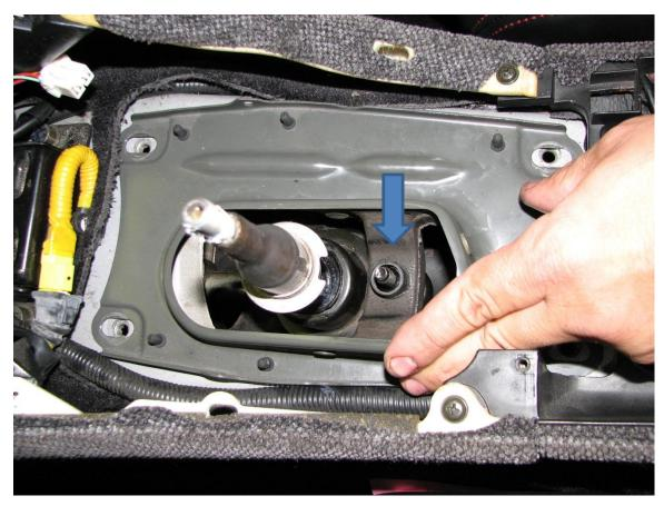
Remove 12mm nut from shift mount rubber mounting point. Then remove stock shift mount plate
